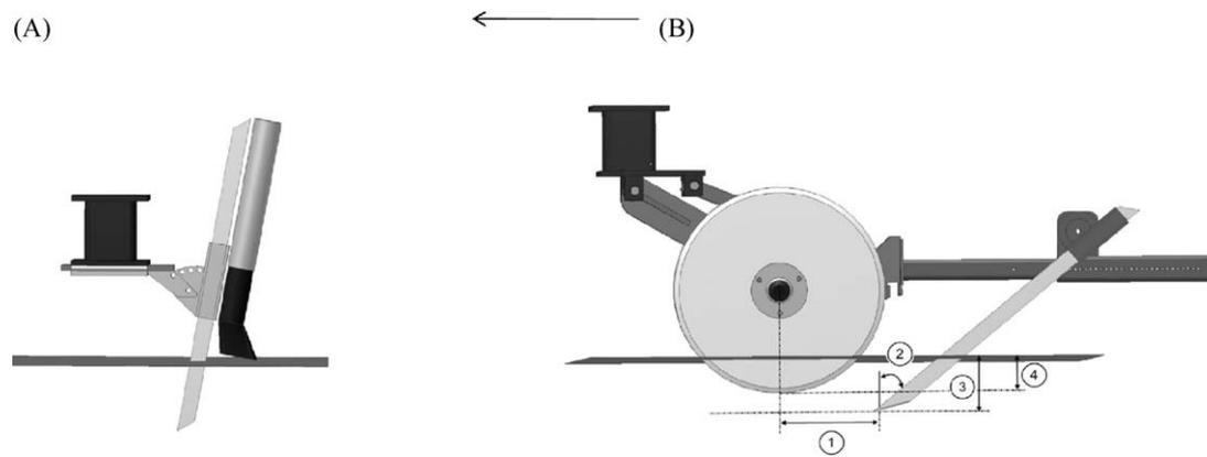
**Fig. 1.** (A) The simple “Agrodan” tine and (B) the experimental slurry injection system, “Bygholm”, used for the study of draught force requirements: (1) distance between discs and tine, (2) 90°-rake angle of the tine, (3) working depth of tine and (4) working depth of discs. Tine operating depth, tine rake angle, distance between tine and discs, and operating depth of discs can be adjusted individually. Array indicates direction of travel.
