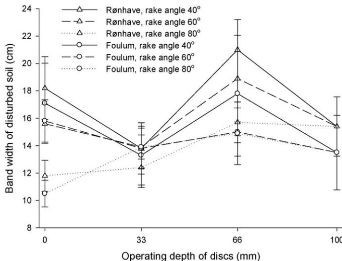
**Fig. 7.** Average bandwidth of the disturbed soil surface across the injection slit, measured for two soils at three rake angles of the tine. For disc operating depths of 0, 33 and 66 mm, the connected tine was operated in the soil bin at 100 mm depth, but an operating depth of 100 mm means that only the discs were running in the soil. Error bars indicate the standard deviation ( $n = 20$ ).
