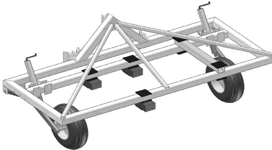
**Fig. 2.** Tractor mounted measuring frame to study the force requirements for the soil-engaging implement, e.g. a slurry injector. The frame is shown with three transducers.
