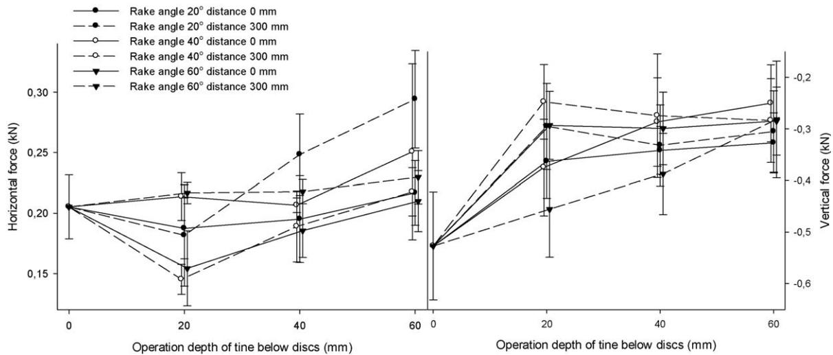
**Fig. 4.** Left panel, average horizontal forces; right panel, average vertical forces. The rolling discs were operated at 40 mm depth and the attached tine was working at three different depths. The simple tine operated at three different rake angles. Only one point is given for operating the tine 0 mm below the discs, since rake angle for the discs are fixed. Error bars indicate standard deviation ( $n = 4$ ).
