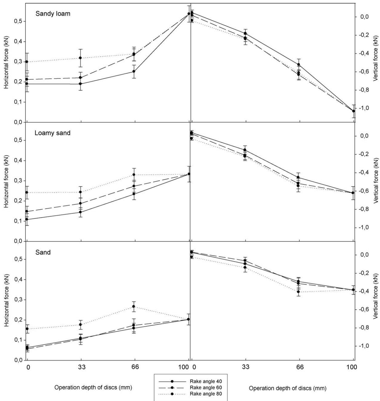
**Fig. 5.** The left column shows average horizontal forces and the right column shows average vertical forces. Measurements were done in three different soil types at four operation depths of the discs. The simple tine operates at 100 mm below the soil surface at three different rake angles except when the discs are operating at a depth of 100 mm, where the tine is not included in the measurements; error bars indicate standard deviation ( $n = 4$ ).
