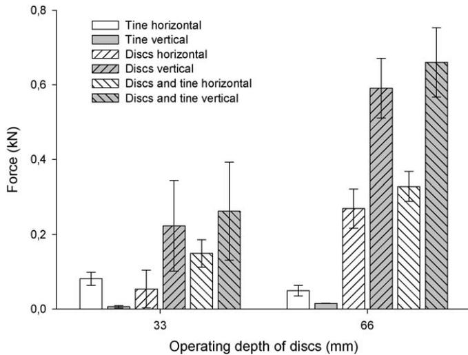
**Fig. 6.** Average force measurements of tine, discs, and the combination of tine and discs; error bars indicate standard deviation ( $n = 3$ ). Tines were operated 100 mm below the soil surface with a rake angle of 60°.
